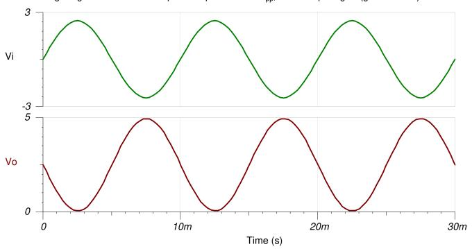
The following image shows the filter output in response to a  $5-V_{pp}$ , 10-kHz input signal (gain = -0.01V/V).
