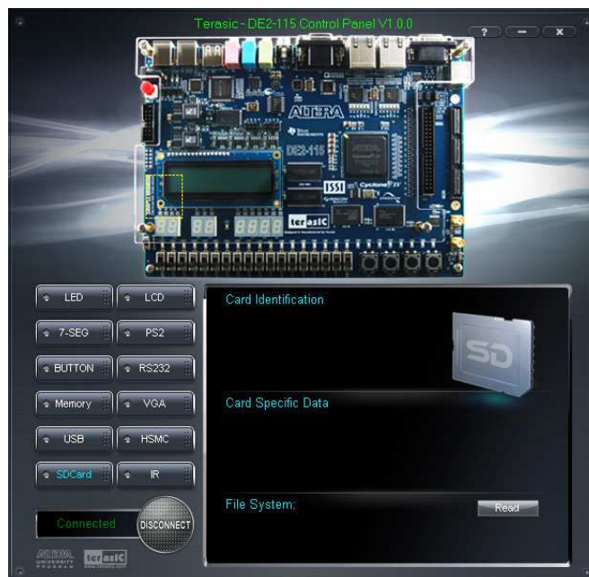
Figure 3-10 Reading the SD Card Identification and Specification
