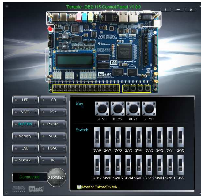
Figure 3-6 Monitoring switches and buttons
