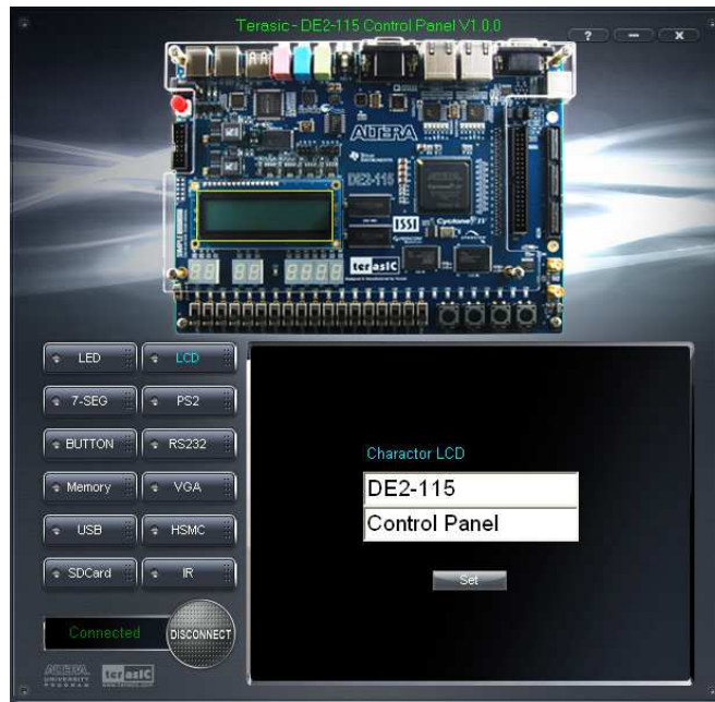
Figure 3-5 Controlling the LCD display
