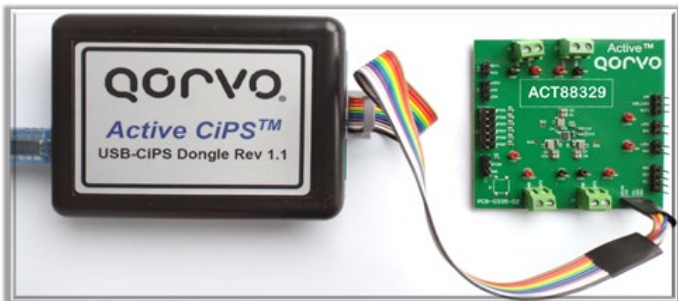
Figure 6: ActiveCiPS™ Dongle enables you to debug your design and change the PMIC default settings on your boards on the spot. (Source: Qorvo).
