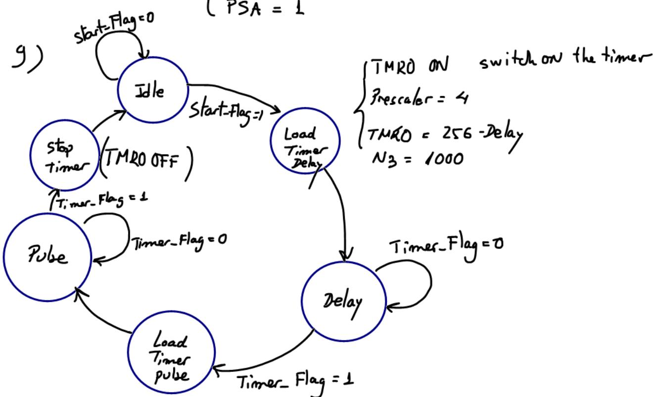
6 states are required to generate the delay and the pulse
