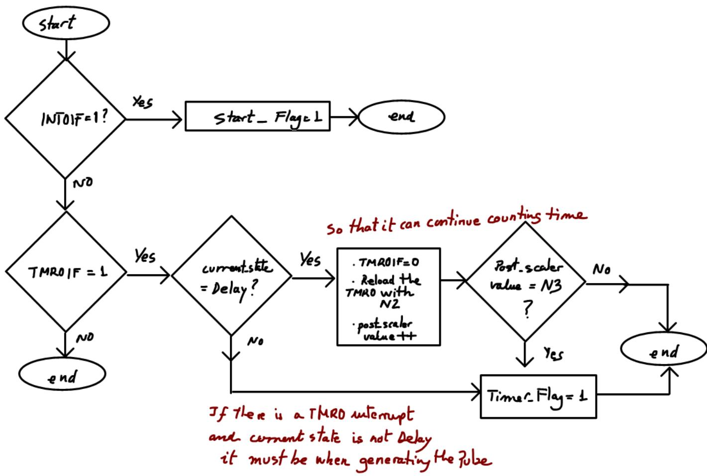
i) output-logic generates the variables Var\_Pulse, Var\_LED\_on and the values to configure the Timer0
