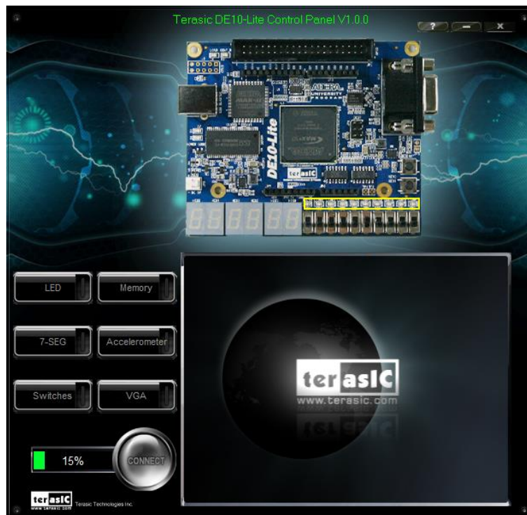
Figure 2-1 The DE10-Lite Control Panel
