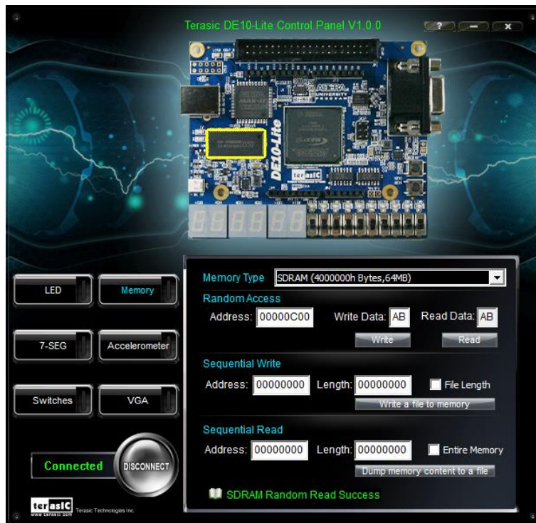
Figure 2-6 Accessing the SDRAM
